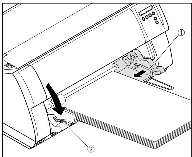
Adjust the right-hand paper guide ① to the width of the paper and move the paper support to the middle of the paper stack. Press down the fixing lever ②.
