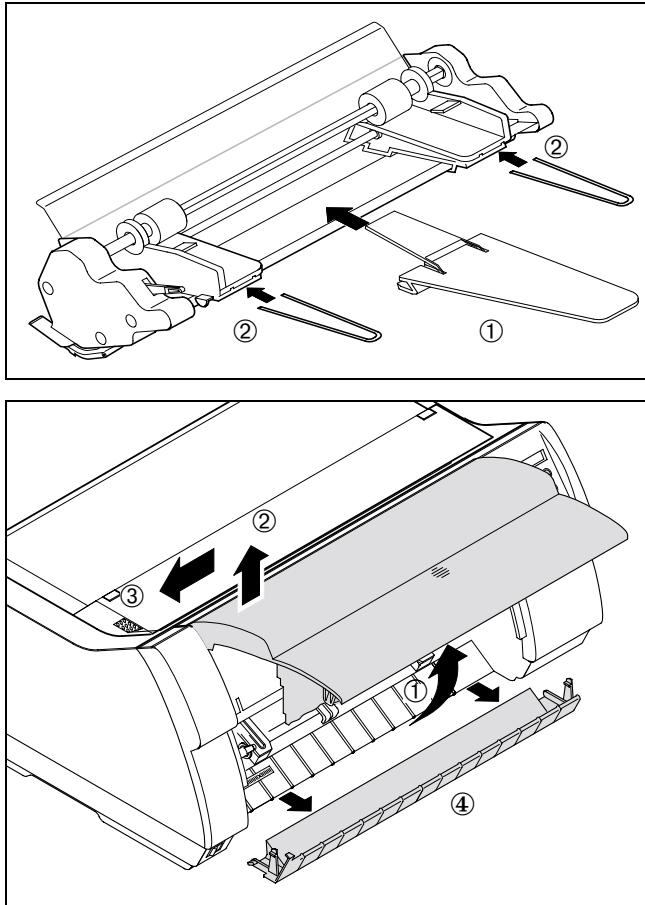
Mount the paper support ① to the holder. Insert the two paper support brackets ② into the openings provided in the paper guides.
