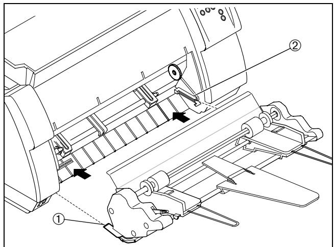
Installation must be performed with the sheet feeder's toothed wheel on the right.
