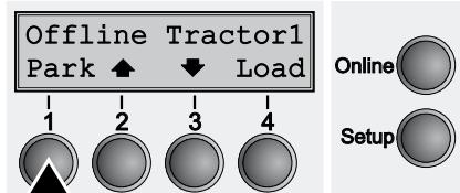
Make sure that the printer is in offline mode; press the **Online** key, if necessary. Press the **Park** (1) key. If fanfold paper is loaded in the printer, it is fed to the tear position. The text **Tear paper off** appears in the display. Then press any key. If a single sheet is loaded in the printer, it is ejected.
